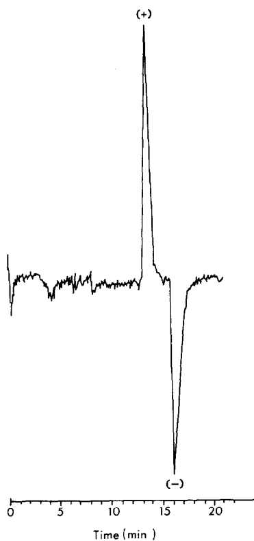
Fig. 3. HPLC separation of diphenyl-ts on (+)-poly(triphenylmethyl methacrylate)-coated silica gel. Mobile phase: methanol at a flow-rate of 0.5 ml/min; ACS ChiraMonitor.
